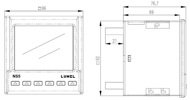
Fig.3. Overall dimensions of NS5 meter
