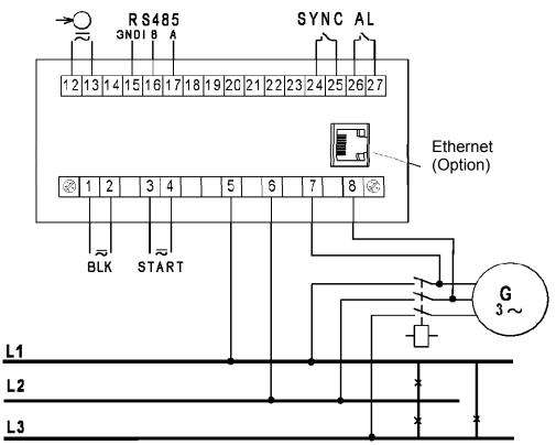
Fig. 4b Connections of the synchronizing unit - phase-to-phase measurement voltages
