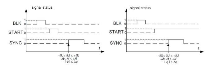
a,b) SYNC relay energized after synchronization conditions are met
