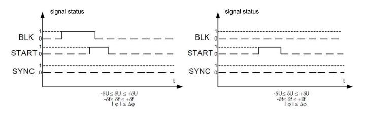
c) **SYNC** relay not energized despite meeting synchronization conditions (START signal blocked by BLK signal)  d) SYNC relay not energized despite meeting synchronization conditions (BLK signal did not change its status from "1" to "0")
